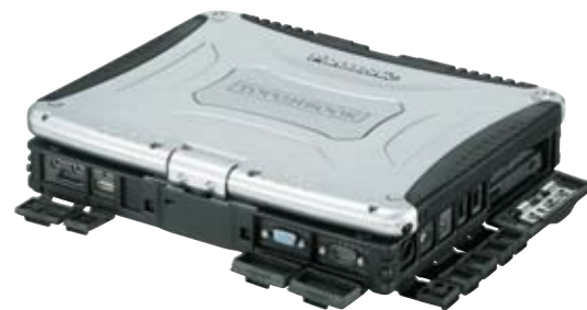
Parts inside the case are enclosed with special waterproof packing and a waterproof sheet, uniformly moulded to each button, covers the keyboard. Also, each cover on the TOUGHBOOK employs a locking mechanism to maintain pressure on the packing when closed.
